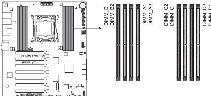
WS X299 SAGE/10G 288-pin DDR4 DIMM socket
